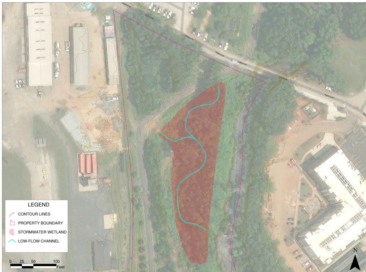
Figure 1.1 - Map of proposed area and stormwater wetland.
