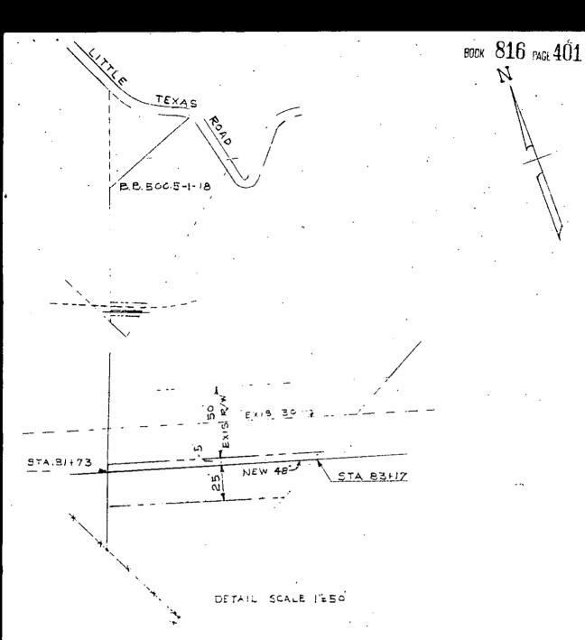
$80\ \text{foot}$  right of way herein conveyed includes existing right of way of 50 feet.
