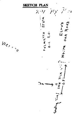
To install 68 ft. of drain tile as indicated above.
