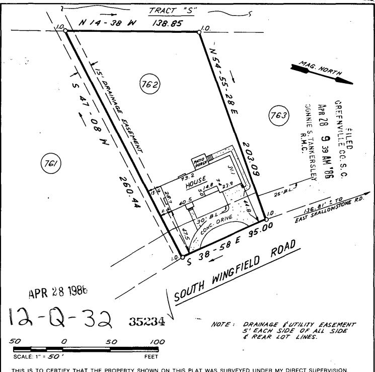
THIS IS TO CERTIFY THAT THE PROPERTY SHOWN ON THIS PLAT WAS SURVEYED UNDER MY DIRECT SUPERVISION. PROPERTY LINES AND IMPROVEMENTS SHOWN ARE LOCATED CORRECTLY AND THAT NO VISIBLE ENCROACHMENTS EXIST UNLESS OTHERWISE SHOWN. THIS PROPERTY IS NOT LOCATED IN A DESIGNATED FLOOD HAZARD AREA.
