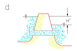
Figure 2 Illustration of drop inlet spillway as a flow control structure: (a) weir control, (b) orifice control, (c) pipe flow with free outfall, and (d) pipe flow with tailwater control.
