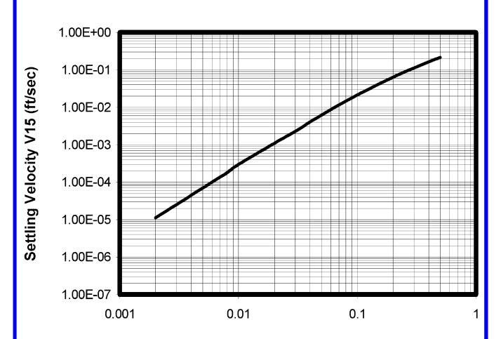
**Eroded Particle Diameter D15 (mm)**
