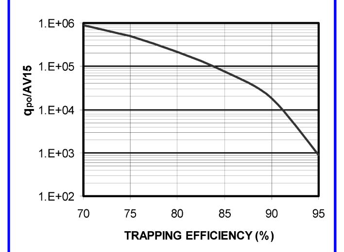
DESIGN AID FOR ESTIMATING TRAPPING EFFICIENCY FOR SEDIMENT BASINS NOT LOCATED IN LOW LYING AREAS AND/OR NOT HAVING A HIGH WATER TABLE
