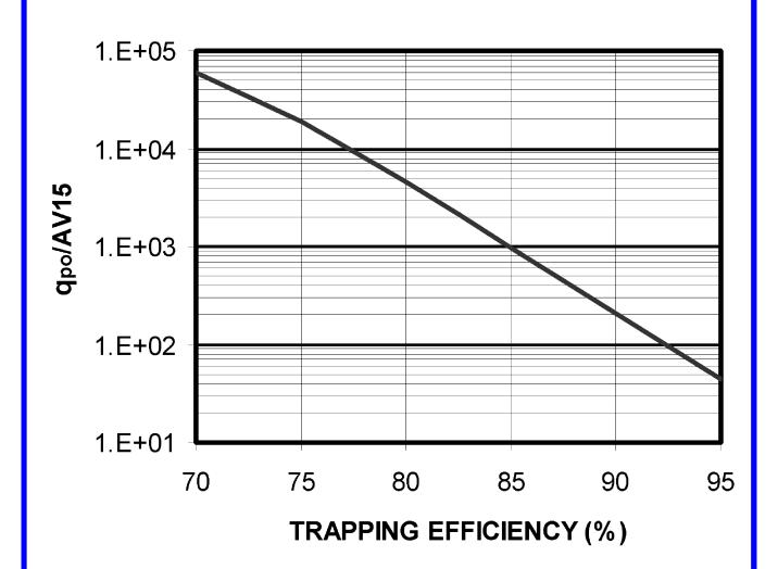
DESIGN AID FOR ESTIMATING TRAPPING EFFICIENCY FOR SEDIMENT BASINS LOCATED IN LOW LYING AREAS AND/OR HAVING A HIGH WATER TABLE
