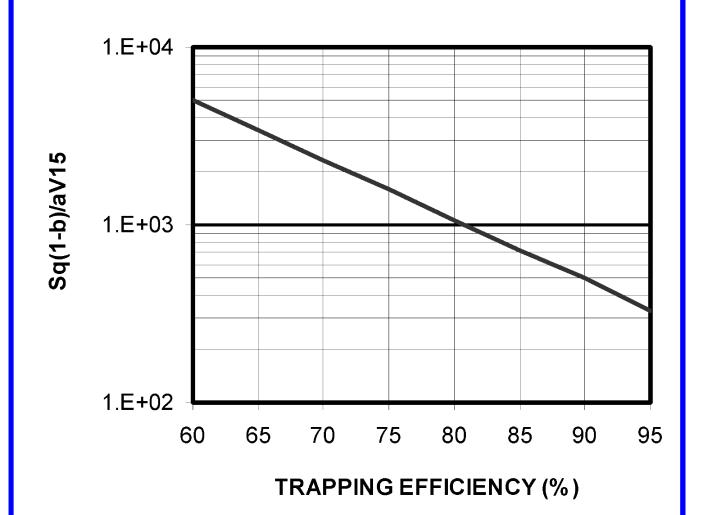
DESIGN AID FOR ESTIMATING TRAPPING EFFICIENCY
