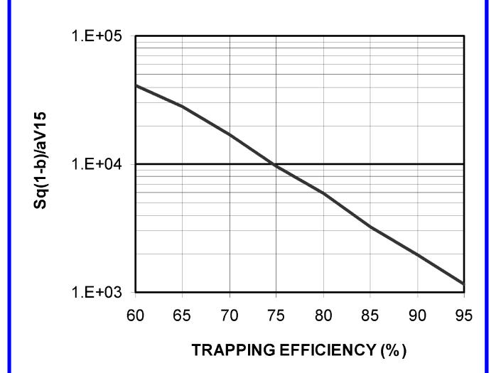
DESIGN AID FOR ESTIMATING TRAPPING EFFICIENCY OF ROCK DITCH CHECKS WITH MEDIUM TEXTURE SOILS
