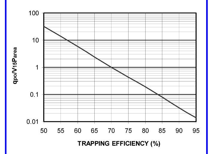
**DESIGN AID FOR ESTIMATING TRAPPING EFFICIENCY OF SILT FENCE**
