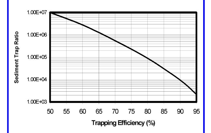
DESIGN AID FOR ESTIMATING TRAPPING EFFICIENCY OF SEDIMENT TRAP
