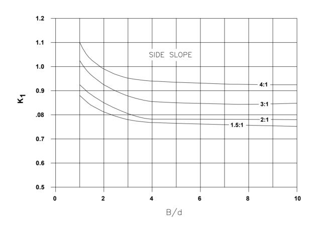
DISTRIBUTION OF BOUNDARY SHEAR AROUND WETTED PERIMETER OF TRAPAZOIDAL CHANNEL
