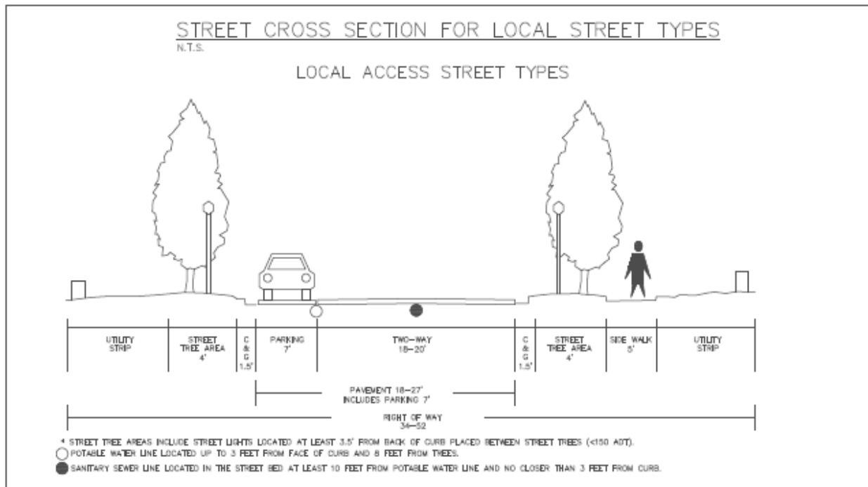
Exhibit 13.1 Street Cross Section for Local Street Types.
