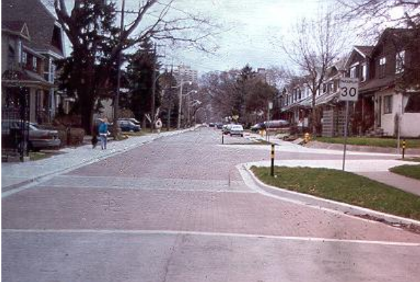
Raised Intersection with Neckdown
