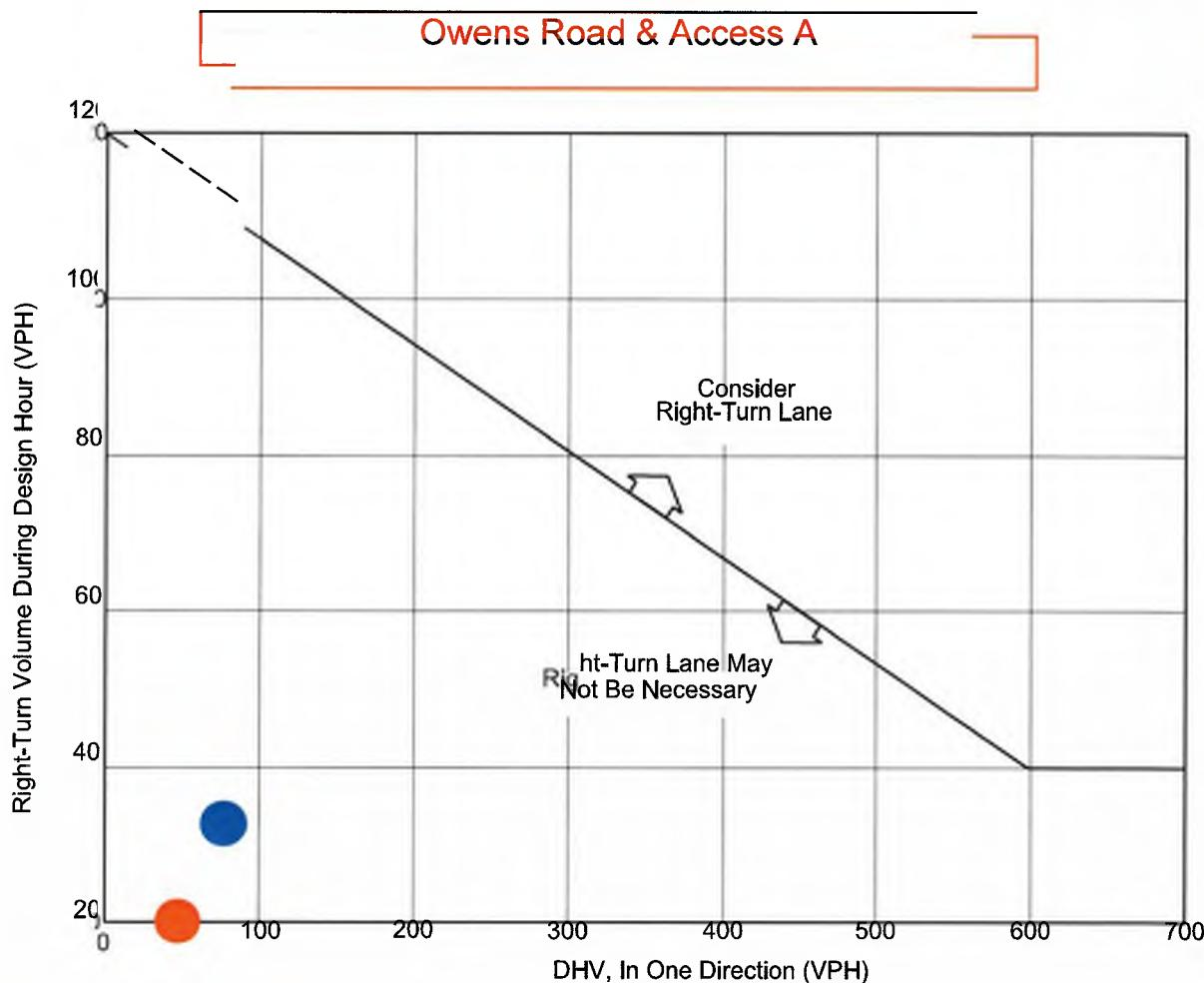
**Note:** For highways with a design speed below 50 miles per hour with a DHV < 300 and where right turns > 40, an adjustment should be used. To read the vertical axis of the chart, subtract 20 from the actual number of right turns.
