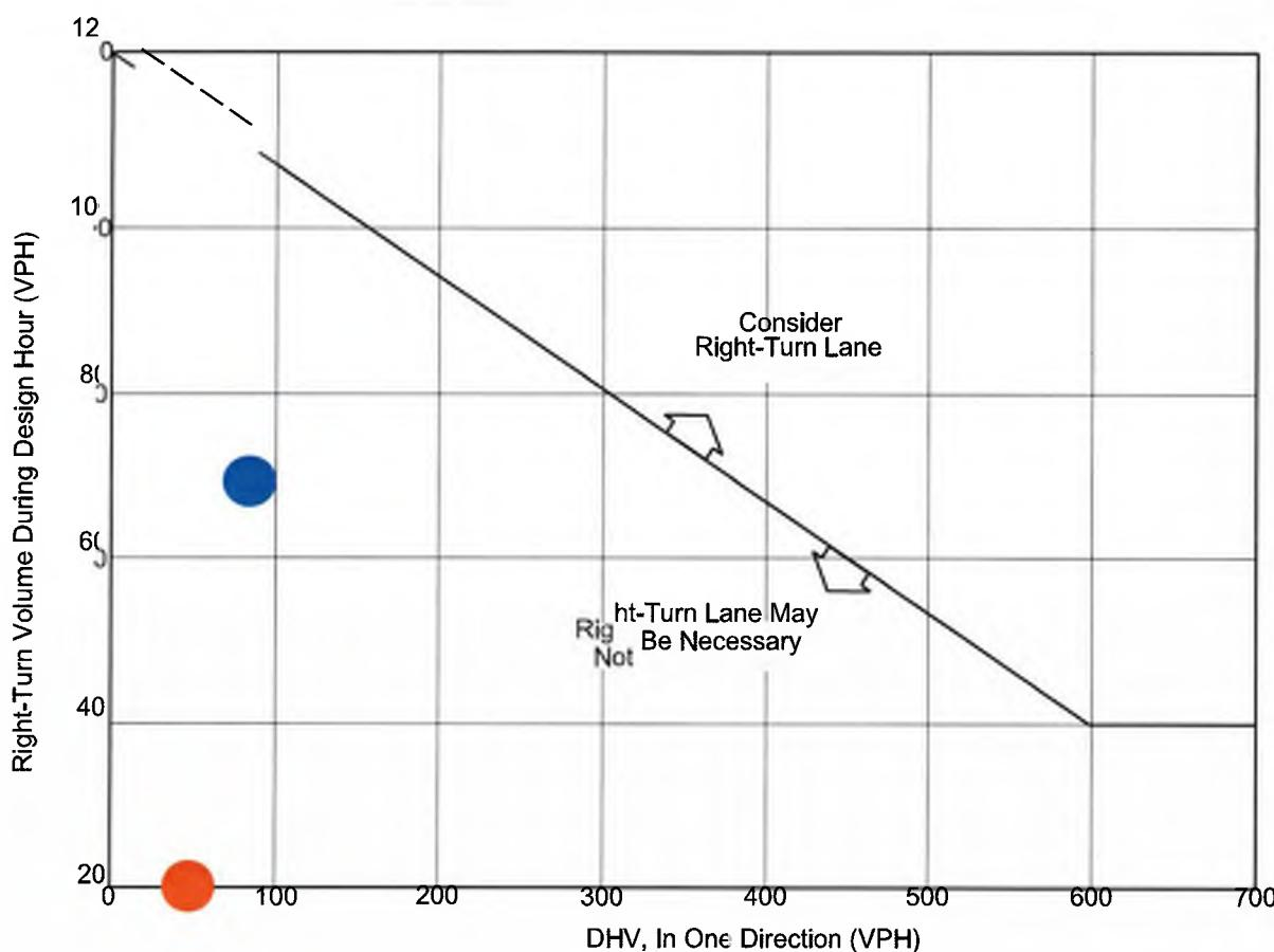
**Note:** For highways with a design speed below 50 miles per hour with a DHV < 300 and where right turns > 40, an adjustment should be used. To read the vertical axis of the chart, subtract 20 from the actual number of right turns.
